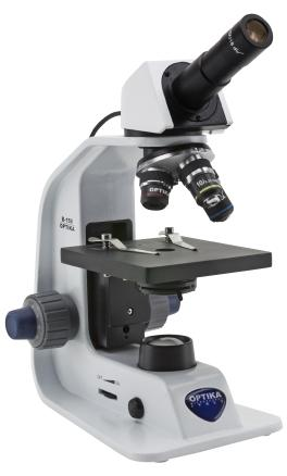
Monocular microscope ideal for students and primary schools, with three achromatic lenses (400x), FN 18 high eyepoint eyepiece, finite optical system, coaxial focusing, fixed stage and powerful, uniform, white color temperature settable 1 W **X-LED**<sup>1</sup> illumination. Slim and easy to carry, the LED illumination will provide over 20 years of use of use. The exclusive ALC will automatically adjust the brightness according to your preferences
