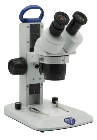
Cordless binocular stereomicroscope ideal for industrial purposes and students/amateurs to dissect and discover mainly biology and materials science in 3D, with turnable objective (2x-4x), FN 21 high eyepoint eyepieces, precision fixed arm with handle and the latest technology of EcoLED™ illumination plus rechargeable batteries. Slim and easy to carry, it is equipped with long lasting LED illumination to provide over 20 years of use
