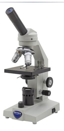
Cordless monocular microscope ideal for students and mainly primary schools, with achromatic lenses (400x), FN 18 eyepiece, finite optical system, coaxial focusing, fixed stage and 0.5 W LED illumination with rechargeable batteries. Slim and easy to carry, it is equipped with long lasting LED illumination to provide over 20 years of use
