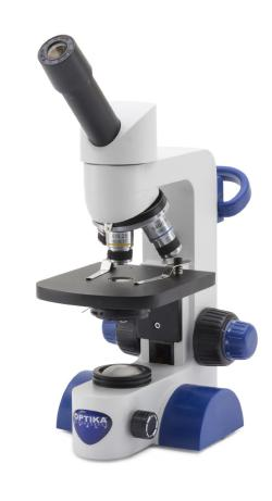
Cordless, modern monocular microscope ideal for students and mainly primary schools with achromatic lenses (400x), FN 18 eyepiece, finite optical system, coaxial focusing, StagErase™ eraseable fixed stage and 1 W LED illumination with rechargeable batteries. Slim and easy to carry, it is equipped with arm/wrist rest support to reduce the fatigue during use and long lasting LED illumination to provide over 20 years of use
