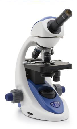
Monocular microscope ideal for teachers and secondary schools, with four N-PLAN objectives (1000x), FN 18 high eyepoint, finite optical system, coaxial focusing, mechanical stage, Abbe condenser and powerful, uniform, white color temperature 3 W X-LED<sup>2</sup> illumination. Slim and easy to carry, yet sturdy and resistant, it is equipped with all the main controls to start learning how to use an advanced microscope and with long lasting LED illumination to provide over 20 years of use
