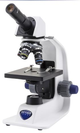
Monocular microscope ideal for students and primary schools, with three achromatic lenses (400x), FN 18 high eyepoint eyepiece, finite optical system, coaxial focusing, fixed stage and powerful, uniform, white color temperature settable 1 W **X-LED**<sup>1</sup> illumination. Slim and easy to carry, the LED illumination will provide over 20 years of use
