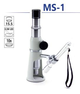
Portable monoscope ideal as multifunctional testing equipment especially for surface analysis and measurements to be used directly on the specimen. Equipped with fixed objective (10x), FN 15.5 eyepiece with crosshair and 0.3 W LED penlight for incident illumination powered by rechargeable batteries
