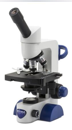
Cordless, modern monocular microscope ideal for students and mainly primary schools with achromatic lenses (1000x), FN 18 eyepiece, finite optical system, coaxial focusing, StagErase™ eraseable mechanical stage, Abbe condenser and 1 W LED illumination with rechargeable batteries. Slim and easy to carry, it is equipped with arm/wrist rest support to reduce the fatigue during use and long lasting LED illumination to provide over 20 years of use
