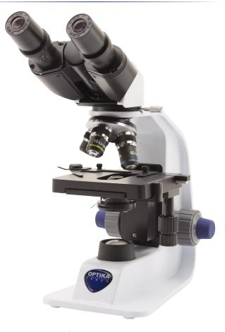
Binocular microscope ideal for students and primary schools, with four achromatic lenses (600x), FN 18 high eyepoint eyepieces, finite optical system, coaxial focusing, mechanical stage, Abbe condenser and powerful, uniform, white color temperature 1 W X-LED<sup>1</sup> illumination. Slim and easy to carry, it is equipped with all the main controls to start learning how to use an advanced microscope and with long lasting LED illumination to provide over 20 years of use
